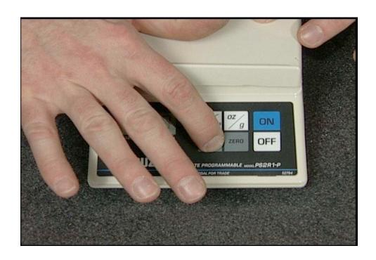
Turn the scale over, press the count key...
